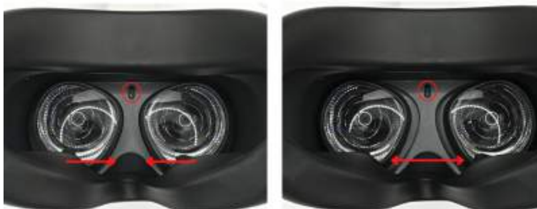
Fig. 5a. Lens-spacing slider inside visor
