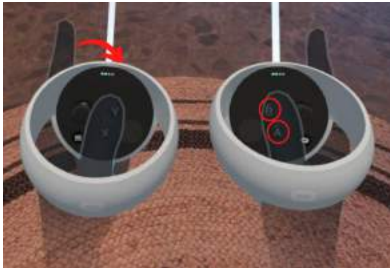
Fig. 2b. Holding controllers with index fingers near triggers and thumbs resting on face buttons ( A and B for Right controller, X and Y for Left controller)
