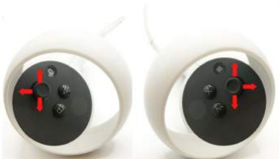
Fig. 4a. Controller analog sticks have 360-degree rotation
